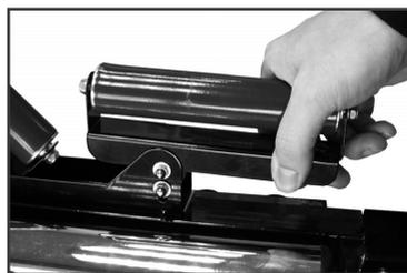
Push down the spring mechanism and tilt the V-shaped Rollers.
